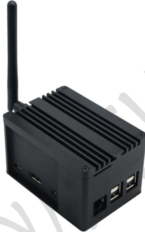
**NOTE: Never power on the gateway without the antenna connected as shown in the picture**
