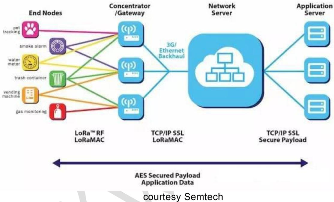
The chart above shows the various parts of Lora's wireless architecture. LoRa network is mainly composed of terminal (built-in LoRa module), gateway (or base station), server and cloud. Application data can be transmitted bidirectionally.
